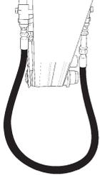
2. Run the hydraulic oil through the carrier's oil filter for approximately 3 minutes to make sure that the hoses are clean.
